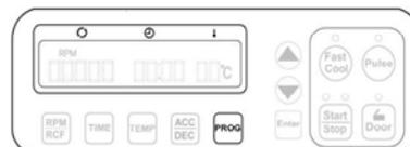
3. Touch the [▲ ▼] buttons to change input Program number. If you do not touch the [▲ ▼] button for 5 second, the setting mode is cleared.
