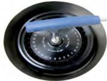
9. To close the rotor lid, rotate the rotor lid nut clockwise. For opening lid: rotate the rotor lid nut counterclockwise.
