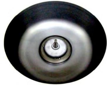
8. Grasp the rotor with one hand, and place Rotor Locking Tool at the center hole of the rotor.
