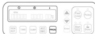
When you touch the [Enter] button, display window shows the saved setting parameters (RPM / RCF, TIME, TEMP).
