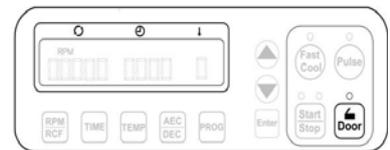
5. When the door is opened, the door LED turns on. When the door is closed, the door LED turns off.
